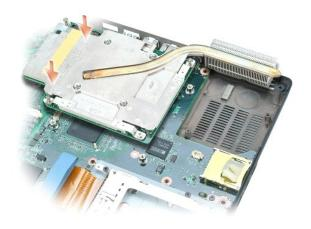
2. Tighten the four captive screws on the video card and thermal cooling assembly.
