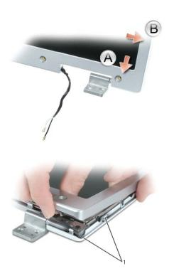
7. Repeat step 6 for the left corner of the bezel. Then use your fingers to release the snaps around the rest of the bezel and lift it away from the cover.
