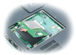
2. Connect the antenna cables to the Mini PCI card.
